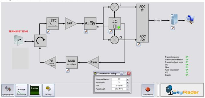
The signal conversion chain of the Pulse Radar Module is like in a real operational radar. Many measurement sockets allow for profound analysis of the signals throughout their conversion with an oscilloscope (not part of the deliverable).
